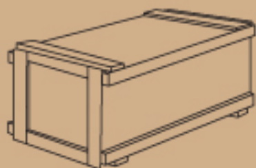
Style E Full cleating on ends, horizontal cleats on sides with top and bottom side to side cleats. Top and bottom fitting between the ends (Lock Corner Cleating).
