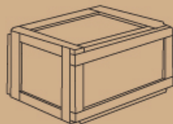
Style B Full cleating with top and bottom fitting between the ends (Lock Corner Cleating).
