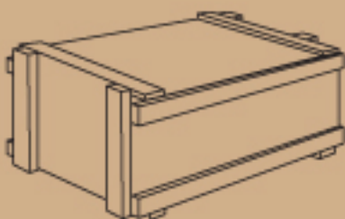
Style D Vertical cleating on ends, horizontal cleating on the sides with top and bottom side to side cleating.
