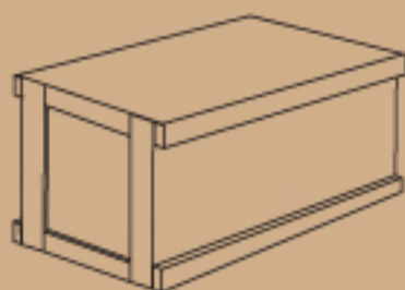
Style C Full cleating on ends, horizontal cleating on the sides with solid panel top and bottom.
